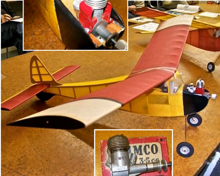
Left: Exhaust deflectors on Keith Trillo's Tomboy, to ensure that oil is directed inside the cowling. See inset.
