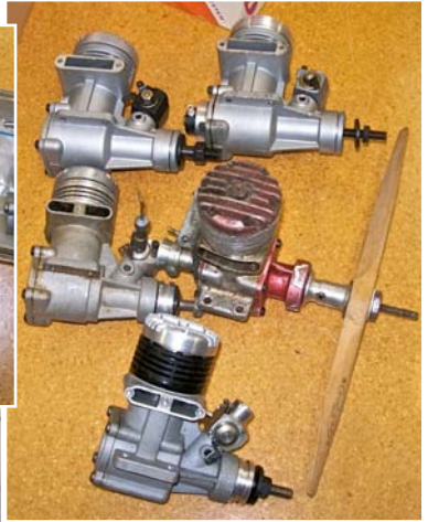
Upper: Engines brought by Arthur Pearce including (clockwise from lower left) a 10cc Pepperell race car glow engine with extended crankshaft modified for aircraft use, .21 Pepperell diesel and Team race diesel, Pepperell 2cc diesel and 19 Spark ignition, two K&B 61s, MkI Merco 61, McCoy 61 and MkII Merco .61 and Eta 29.
